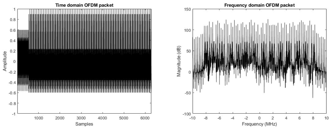
**Figure 4: OFDM packet used in our testing setup. There are 8 preamble symbols, each with the bit sequence 01-10010101-11110011-01010000-00110010-10000001-10010100-00. There are 72 data symbols, each with the bit sequence 10001111-11110001-11111100-01111001-10011011-11100000.**
