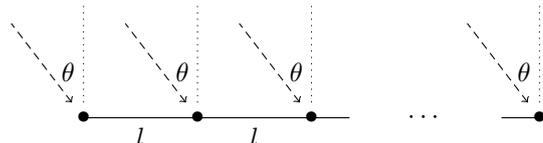
**Figure 2:** The received signal (dashed) angle  $\theta$ , relative to the vector perpendicular to the array, is approximately the same per-antenna (dot).
