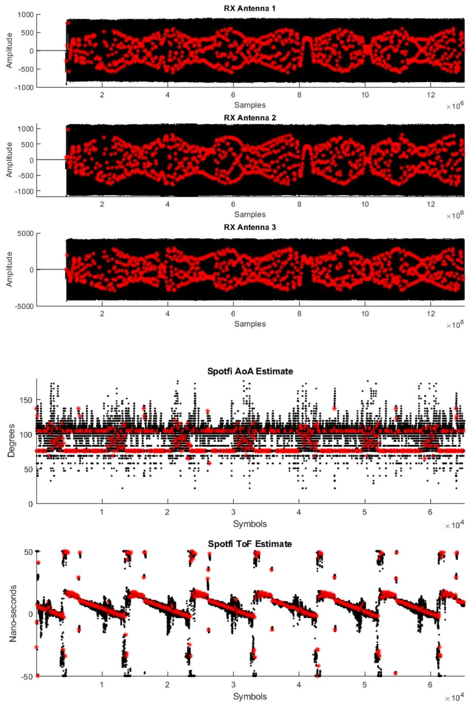
Figure 8: Same setup as before, but signal arrives at 113 degrees at distance about 115 centimeters. This test was ran for 30 seconds (the first 15 being lost), and thus yielded significantly more data. The AoA estimate here fluctuates between about 75 degrees and about 104 degrees. Notice that each preamble-computed channel is roughly the same for each cycle, but the individual data symbol channels are slightly different.
